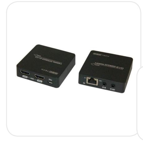
HDMI signal extender over Ethernet cable (cat 6) to transfer HD 1080p signal up to max 55 m without loss of signal and quality, with second through HDMI port and remote control repeater.
