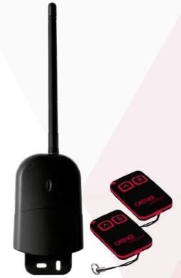
Frequency Type of coding Number of channels Installation Use Programming Relay Memorised codes Power supply Batteries Degree of protection Operating temperature 433,92 MHz Fixed 2 configurables: monostable/bistable Outdoor Gates, shutters, boxes, lighting, irrigation Self-learning 12A - 14Vdc - 7A - 120Vac 140 12Vdc - 24Vac 2x 3 V - CR2016 (included) IP 55 -20/+50 °C
